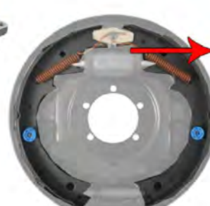
Duo-Servo Larger Shoe Lining to Rear (Left Shown)
